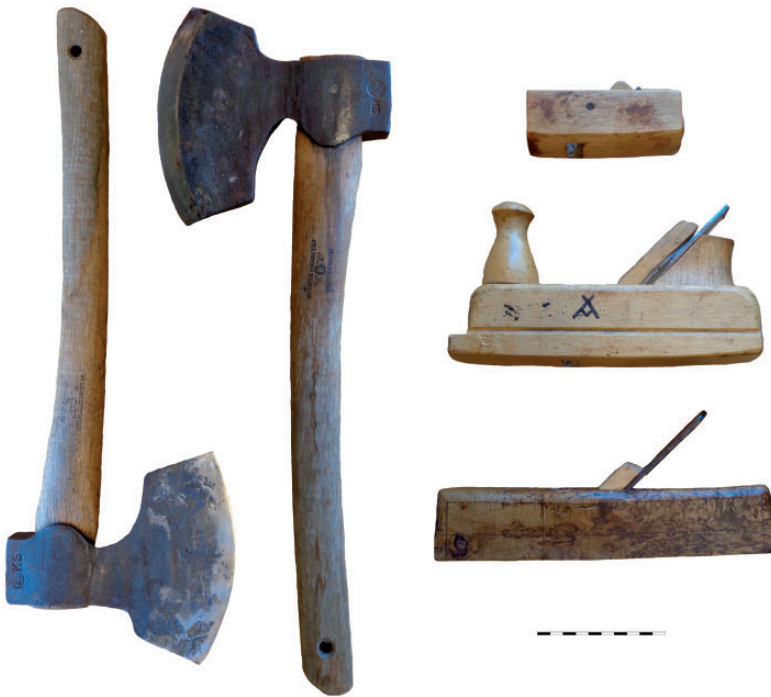
Figure 3. Hand tools used during the construction of the boat. From left to right: two wood working axes; three planes of various sizes. Scale length is 10 centimeters.
